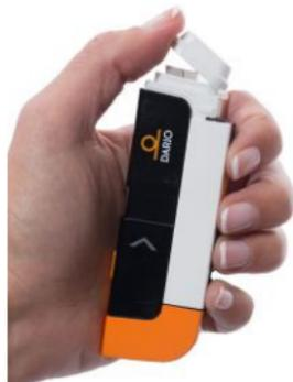
2. Snap open the test strips cartridge cap by pushing up the edge.
